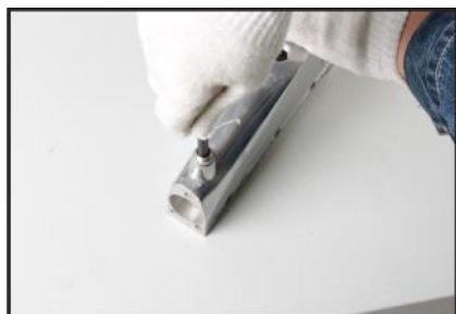
4. Screw coil into casting.
