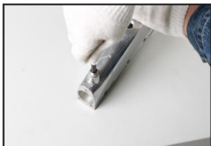
4. Screw coil into casting.
