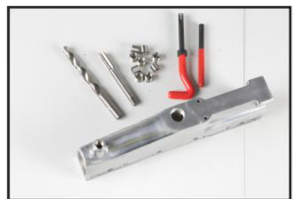
6. Thread is repaired and ready to use.
