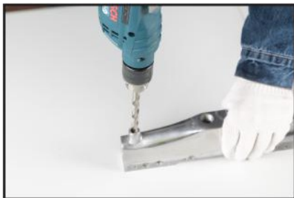
1. Drill out damaged thread using correctly sized drill.
