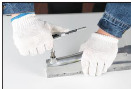
2. Tap re-drilled hole using tap supplied.
