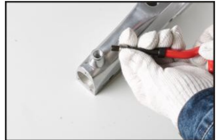
3. Load coiled insert into applicator.
