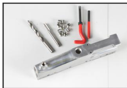
6. Thread is repaired and ready to use.
