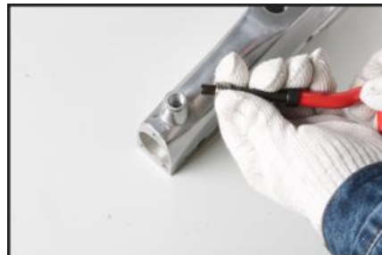
3. Load coiled insert into applicator.
