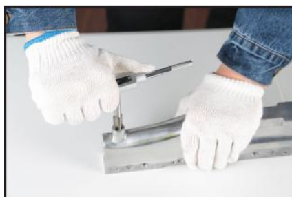
2. Tap re-drilled hole using tap supplied.
