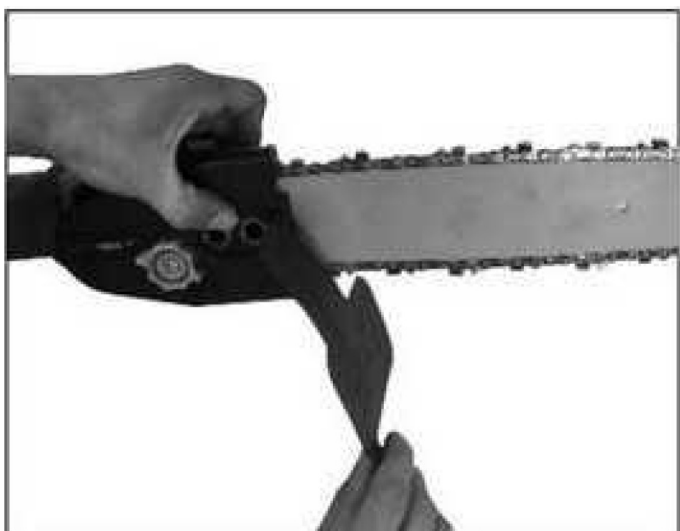
10. Replace the screws, but do not tighten them completely
