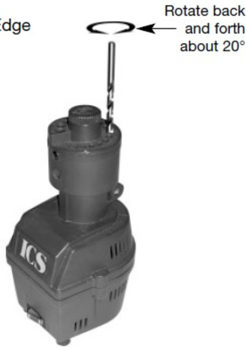
Figure 2 - Putting Bits into Sharpener
